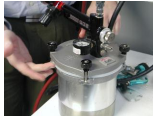
A pressure pot, rather than a gravity feed or siphon setup is the preferred equipment.
