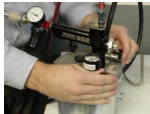
A pressure pot equipped with regulator valves to control air intake and pot pressure.
