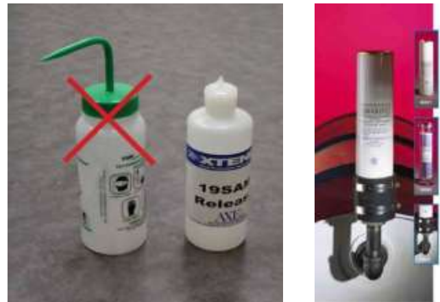
Desiccant drum driers and appropriate bottles will conserve solvent-based semi-permanent mold releases.
