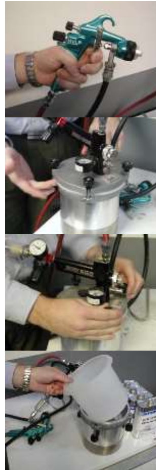
A Binks HVLP equipped with a fluid tip ranging from 1.0-1.8 mm
