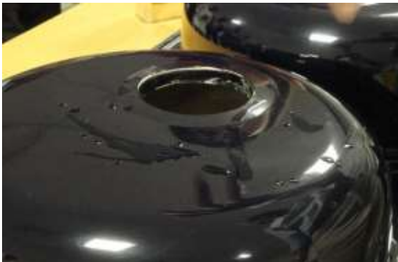
Water droplets that flatten out on the mold surface rather than forming a tight bead, indicate a cleaner surface.
