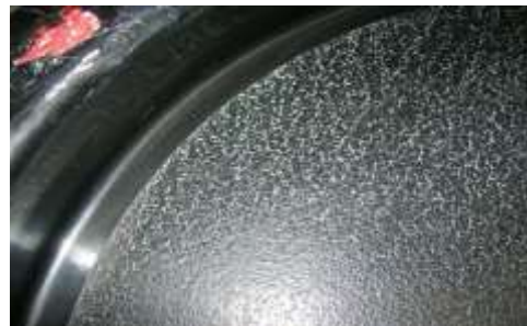
A mold with heavy styrene buildup in the non-skid areas.
