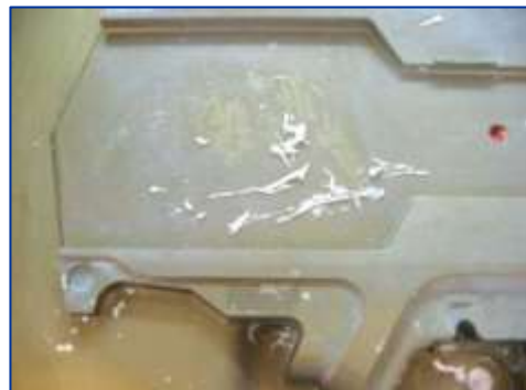
A mold with buildup from too much mold release
